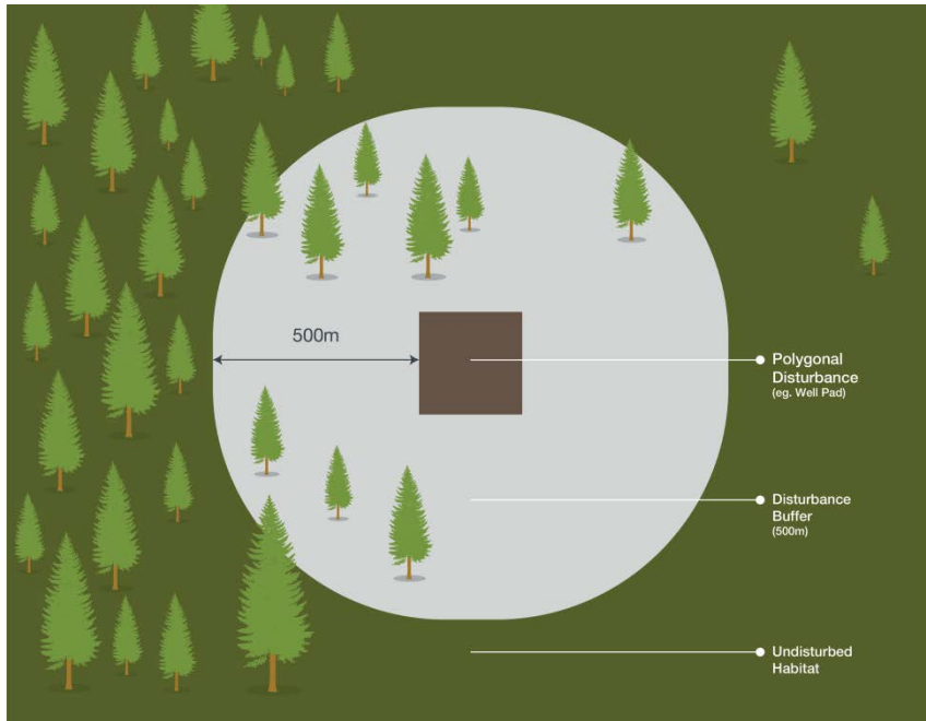
Figure 5 Illustrates how the 500m buffer applies to an area feature like a well pad
